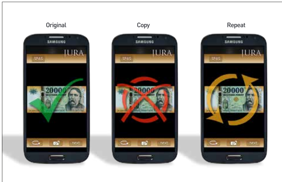
Jura engineered intaglio-printed line feature for authentication by a smartphone.
